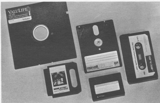
In the middle is the Maxell 3" diskette. Other recording media include 5 1/4" diskette, ROM cartridge, Wafadrive cartridge, and regular cassette tape.
